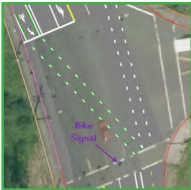
◀ *N Going St: Cyclists will move diagonally across the intersection with a new bike signal.*
